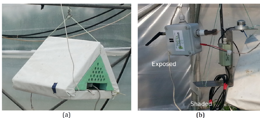
Figure 1. Wireless sensor nodes inside the greenhouse in (a) “boxed” setup and (b) “exposed” and “shaded” setups.
