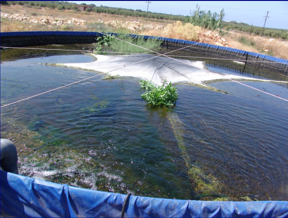
Upper surface of a sand filter
