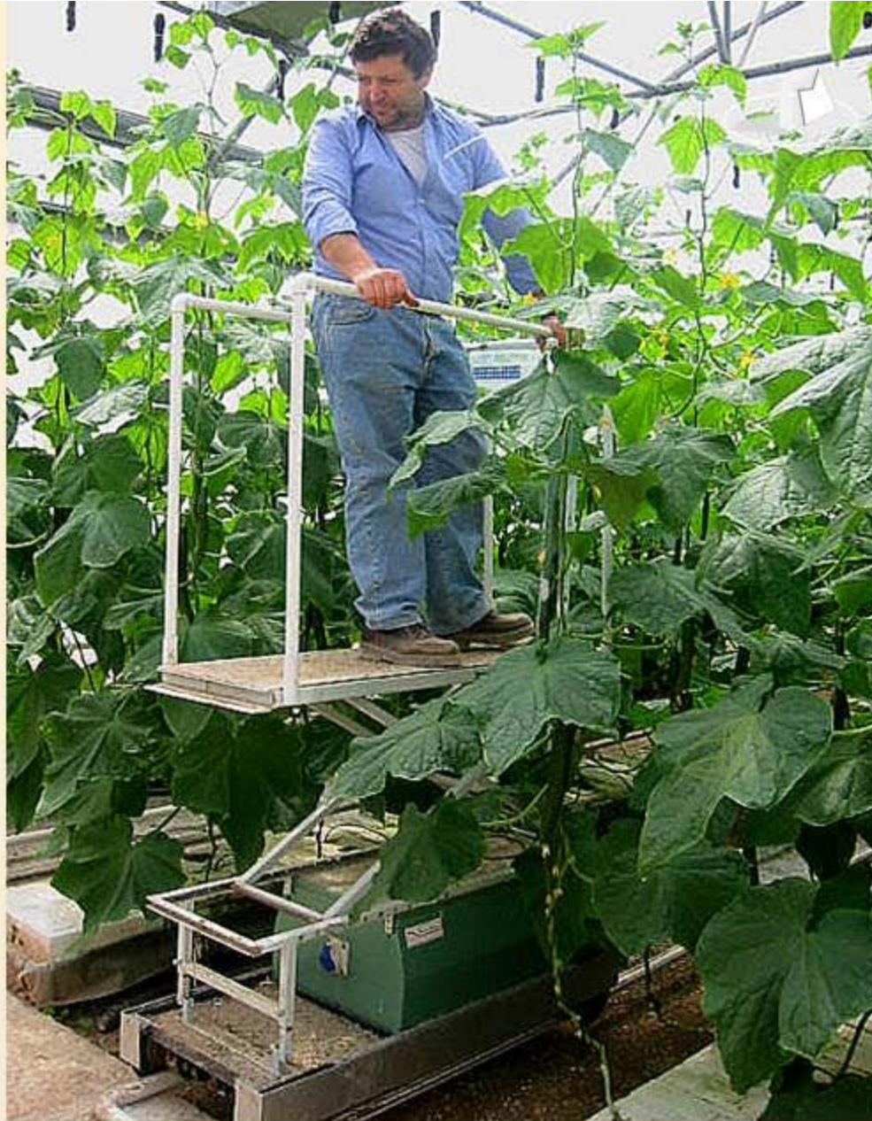
Electric trolley moving on heating pipes
